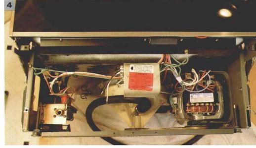
er supply is going to be a line cord with a plug, it is awfully nice to have enough cord to plug into the outlet and still have your machine totally out of the enclosure. Because you have to provide this cord, you can select its length. Now is the time to thread the cord through the hole in the cabinet.
